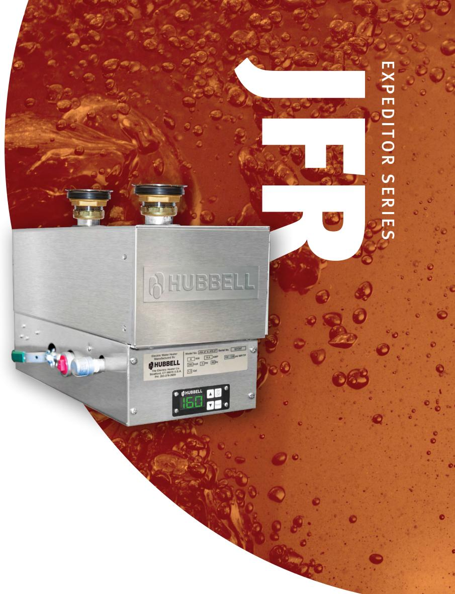
The Hubbell model JFR is designed to heat or hold food at safe serving temperatures when used with a food rethermalizer or bain-marie. Mounted under a holding vessel and typically set between 140°F and 190°F, the Hubbell model JFR provides continuously circulated hot water to efficiently satisfy safe serving requirements and prevent cold spots.
